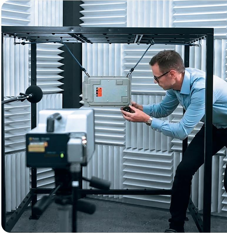
Above: Rickard Jonasson, NVH Engineer adjusting the laser vibrometer for testing.
